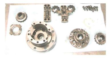
6) After all the parts are clean you will need to chamfer the spring holes on both upper and lower clutch members to remove the sharp corners. This is important to keep the sharp corner from wearing into the new springs. A rotary grinder works fine for this. Also, remove any nicks or burs on the main housing and upper cover using a flat file.
