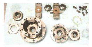
22) It's now time for final assembly. Reinstall all the parts in order just as you did in the above instructions. Make sure you align the match marks on the upper and lower clutch members. Install the MAXGRIP springs and the pinion gears at this time. You need to oil every part during installation. Use the same oil you will be using as your gear lube.
