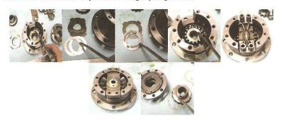
23) Because the MAXGRIP springs are longer and stiffer than the o.e.m. springs, you will need to clamp the upper member to get the pinion gears down into the casing. This will allow you to place the thrust washer onto the upper clutch member. Once the washer is in place you can remove the clamps.
